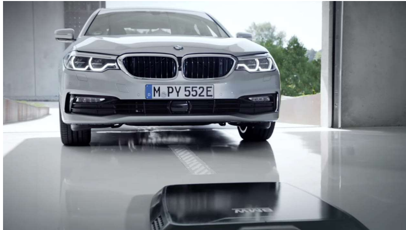
Figure 31: Wireless Charging Pad & EV (Auto Express, 2018)
